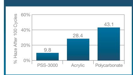
This chart compares increase in haze on 3.0 mm thick sheets after 100 cycles using a CS-10 wheel with a 500 gram weight at 72 rpm per ASTM D1044 and ASTM D1003-07. (Tested by Intertek)
